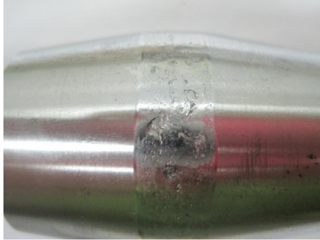
Figure 3 Pitting observed on hardened specimen of first generation RCF tester
