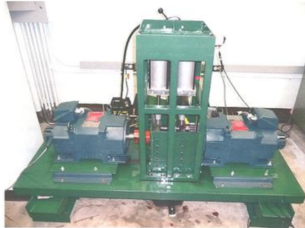
Figure 4 First generation sliding rolling contact fatigue tester [10]
